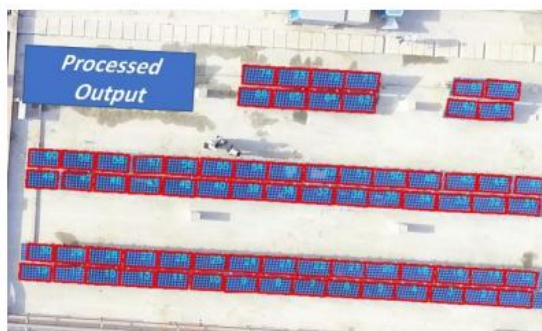
Fig. 7. Aerial Image two after processing from the Raspberry Pi
