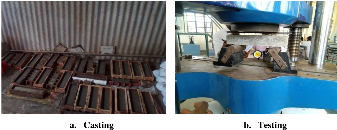
Figure 1. Fibre Reinforced ECC-MS Prism Specimens
