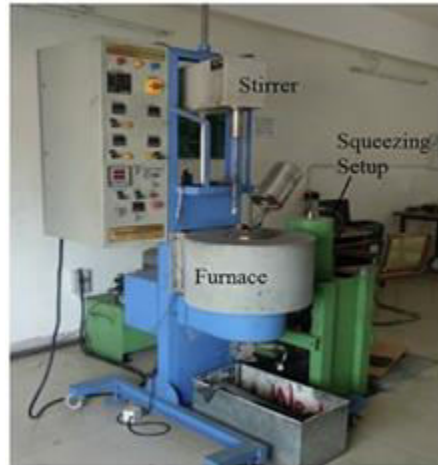
Fig. 1. Squeeze casting setup for MMC processing.
