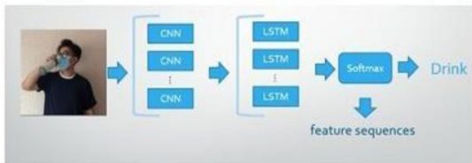
Fig.1 The structure of CNN+LSTM algorithm
