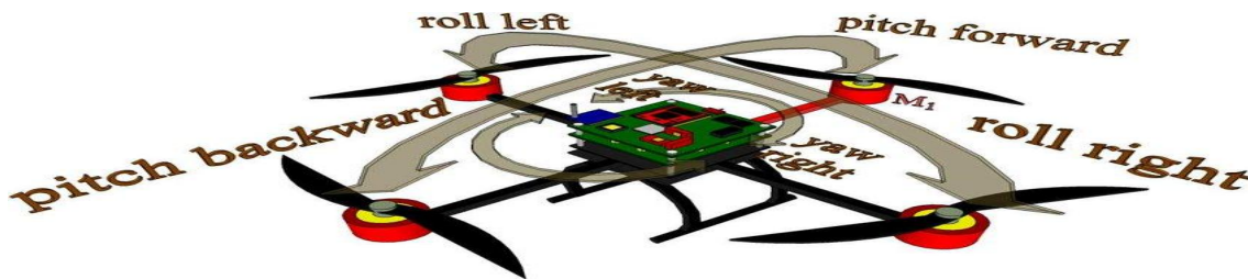
FIG 4.3.2 MOTORS MOVEMENT OF ALL DIRECTIONS INCLUDING PITCH AND ROLL
