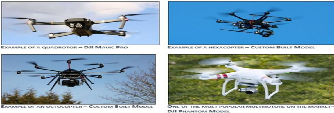
FIG 2.2.1 TYPES OF DRONES BASED ON NO OF ROTORS
