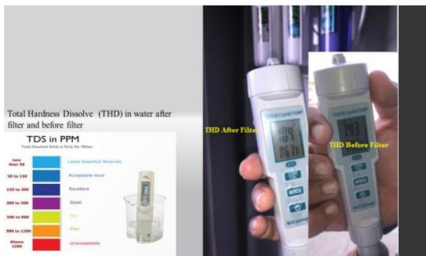
Figure 10. THD after filter and before filter.
