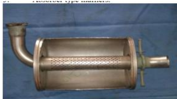
Fig 4: Exhaust Muffler of TATA INDICA CAR Purpose of Muffler
